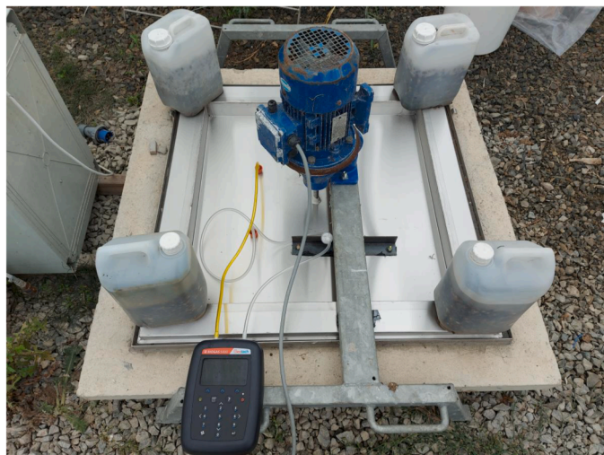
Fig. 1. Stainless-steel lid covering slurry storage prior to agitation during mesoscale incubation. Biogas analyser present in the bottom left. Agitator present in centre of image.
